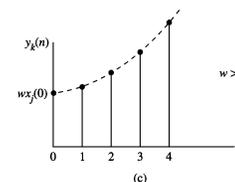
$y_k(n) = \sum_{l=0}^{\infty} w^{l+1} x_j(n - l)$ , so  $w$  determines the behavior. With a fixed  $x_j(0)$ , the output  $y_k(n)$  either converges or diverges.
